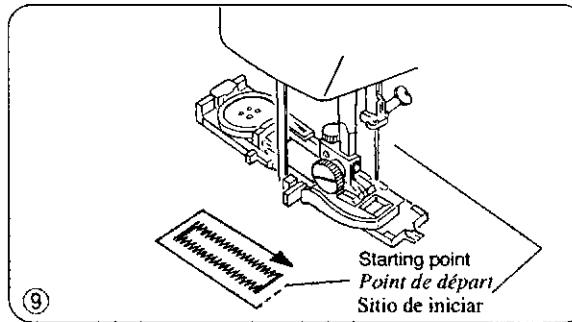
⑨ Sew slowly and stop the machine at the starting point when a buttonhole is completed.
