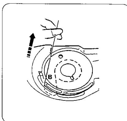
Continue to draw the thread lightly until the thread slips into notch **B**.
