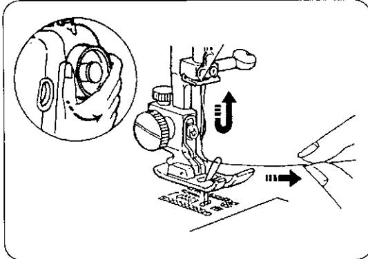
② Turn the balance wheel slowly towards you with your right hand until the needle goes down and continue turning balance wheel until the take-up lever is at its highest position. Lightly draw up the needle thread forming a loop of the bobbin thread.
