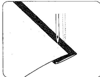
Position the fabric on the machine so that the needle just pierces the folded part of the fabric when the needle comes over to the extreme left side.
