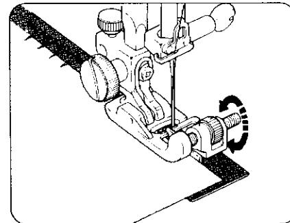
Turn the guide screw and move the sliding guide next to the folded edge.
