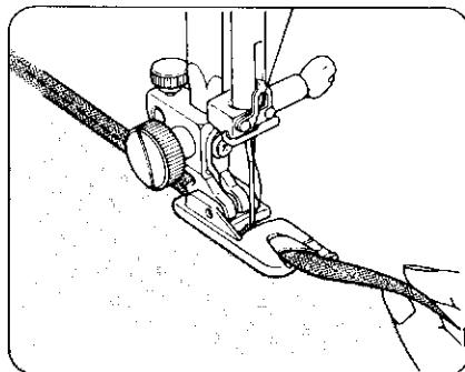
Lower the hemmer foot, then sew by lifting up the edge of the fabric to
