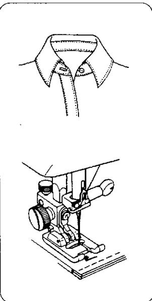
Face the thick stepped part this side and use the buttonhole foot (B) when holing a buttonhole at the edge of a portion where outlet seams overlap each other.
