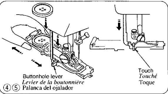
④ Pull the button holder to the back, and place the button in it. Push back the button holder toward you as far as it will go.
