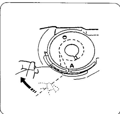
Guide the thread into the notch **A** on the front side of the bobbin holder.
