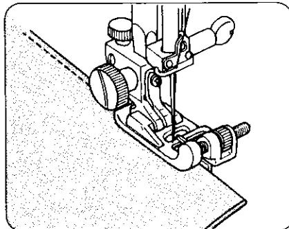
Position the fabric so that the needle pierces 0.1 to 0.2cm(1/16") inside of folded part and lower the presser foot.
