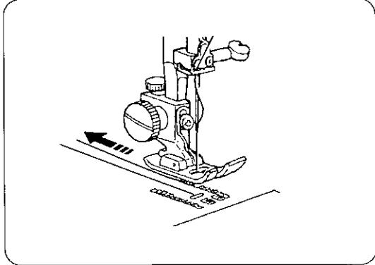
③ Pull 15 cm (6'') of both threads back and under the presser foot.
