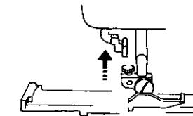
⑬ When buttonhole sewing is finished, push the buttonhole lever upward as far as it will go.
