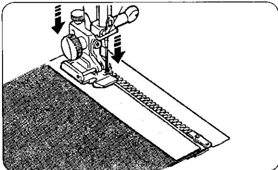
Attach the zipper foot with the pin on the right hand side.
