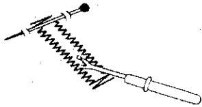
⑩ Cut the both needle and bobbin threads leaving about 10 cm (4") thread ends.
