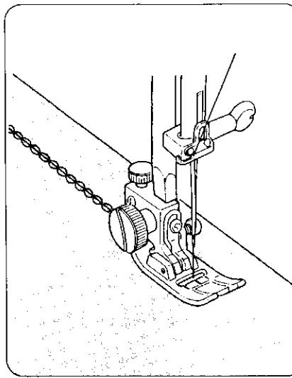
The stitch is sewn with two stitches forward and one stitch backward forming a seam that does not rip easily.
