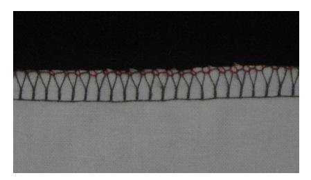
**Fix:** Turn the tension of the upper looper to a higher number of one. Test the seam and if necessary, continue adjusting the tension so that the hitch line falls at the edge of the seam.
