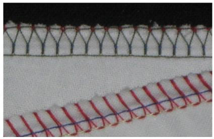
**Fix:** Ajusting only one tension at a time, turn the tension of one of the loopers to a lower number by one. Test the seam and then adjust the tension of the second looper. Continue adjusting the tensions until the seam lays flat.
