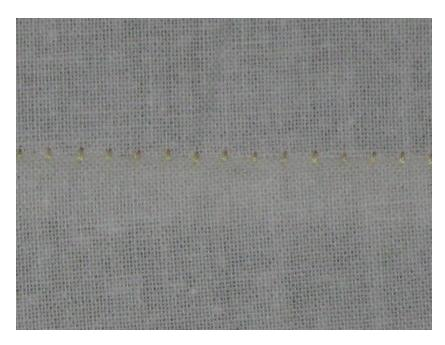
**Fix:** Turn the tension of the right needle to a higher number by one. Test the seam, if necessary, continue adjusting the tension until no thread shows when the seam is opened.
