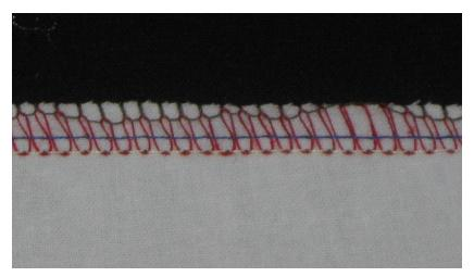
**Fix:** Turn the tension on the lower looper to a higher number by one. Test the seam and if necessary, continue adjusting the tension so that the hitch line falls at the edge of the seam.
