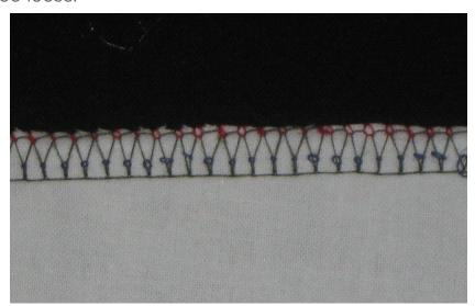
**Fix:** Turn the tension of the right needle to a higher number by one. Test the seam and if necessary, continue adjusting the tension until the loop disappears on the back side of the seam.
