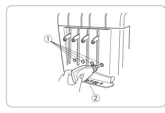
Apply a few drops of oil to the needle bar through the holes in the front cover.
