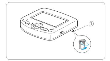
If you are using the RCS unit on the tabletop, simply insert the connector into the connector socket on the back of the machine.
