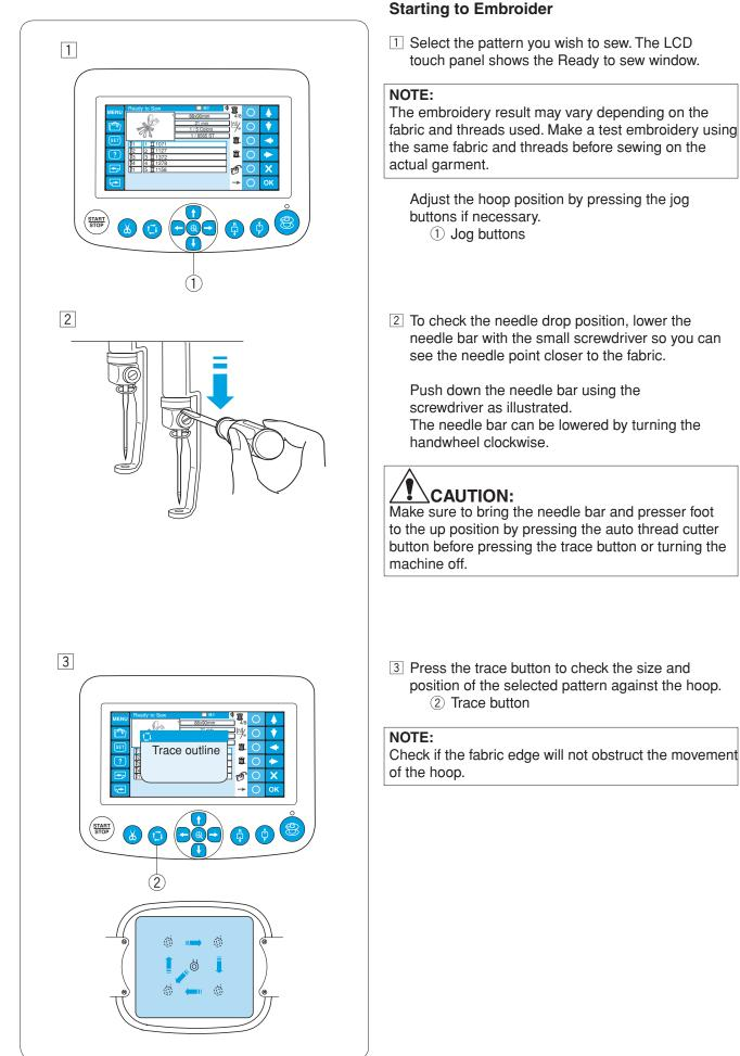
needle bar with the small screwdriver so you can see the needle point closer to the fabric.
