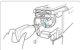
Open the hook cover and remove the bobbin case. Clean the inside of the hook with the lint brush. ③ Hook race
