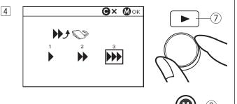
4 Press the right arrow key to enter the desired setting. Turn the either of the jog dials to move the cursor and select the desired setting.
