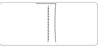
These are narrow stretch stitches designed to eliminate puckering on knit fabrics and bias seams, while permitting the seam to be pressed completely open flat.
