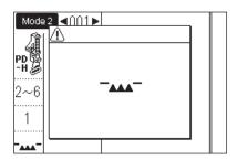
If you start the machine with the feed dog lowered, a message will appear on the LCD screen.
