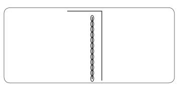
This strong, durable stitch is recommended for areas where both elasticity and strength are needed to ensure comfort and durability.
