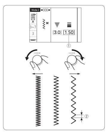
Zigzag stitch is used for various sewing needs including overcasting. It can be used on most woven fabrics. A dense zigzag stitch can also be used for applique.
