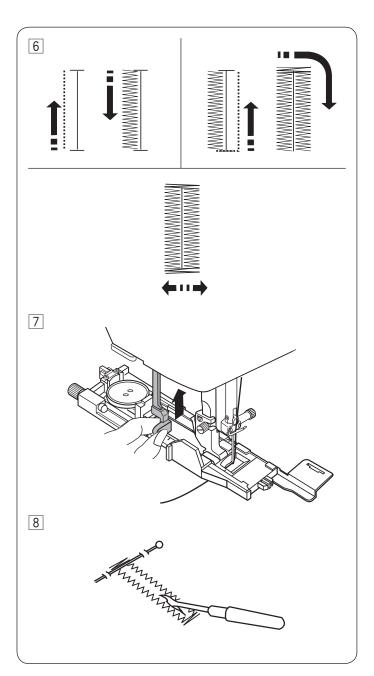
6 The buttonhole is sewn automatically in the sequence shown. When the buttonhole is finished, the machine will stop automatically with the needle in the up position. Press the thread cutter key and remove the fabric.
