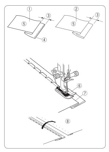
Select pattern 018 in mode 2 for woven fabrics or pattern 19 in mode 2 for elastic fabrics.
