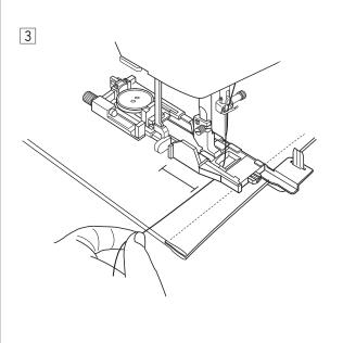
3 Place the fabric between the buttonhole foot and stabilizer plate. Lower the needle into the starting point by turning the handwheel.
