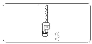
This stitch can be used to simultaneously seam and overcast edges of fabrics.
