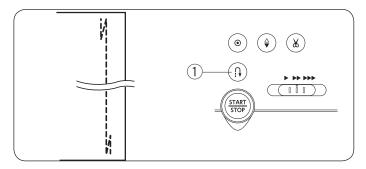
Use this stitch to secure the beginning and the end of a seam with backstitching.
