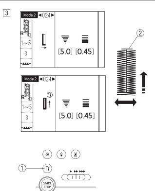
3 Start sewing again, and the machine sews the front bartack and right side of the buttonhole. Stop the machine when you reach the ending point 2. Then press the reverse key 1.
