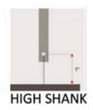
Other ruler feet brands may work on Janome machines, but Janome feet offer easy adjustment of the foot height without tools. Janome feet can be adjusted manually or electronically. It is essential that the foot "kiss" the fabric sandwich when doing rulerwork, so this is a convenient feature of Janome rulerfeet.
