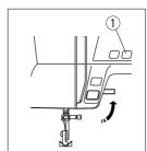
Raise the presser foot. Press the needle up/down button ① to raise the thread take-up lever to its highest position. ① Needle up/down button
