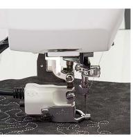
The A.S.R. foot holder reacts to the movement of the fabric and provides the same stitch length for free motion, ruler work, or variable zig zag. We recommend thinking of this system as Free Motion Quilting (FMQ) training wheels. Training wheels that
