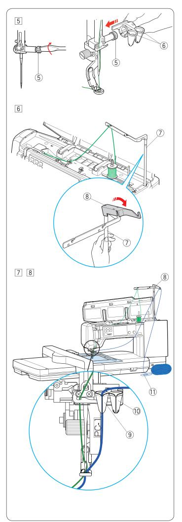
5 Retighten the needle clamp screw firmly with the screwdriver.
