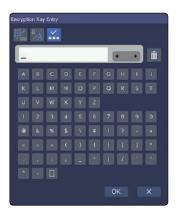
If the selected wireless network requires an encryption key for connection, the Encryption Key Entry dialog box appears. Be careful to enter uppercase or lowercase letters as required.
