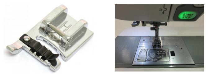
The Satin Stitch Foot F is a great foot to use for decorative stitches and other stitches that are heavier. This foot also provides a little extra room underneath to allow easier passage for thicker materials that may not fit through the small guides on Foot H like bulky cording, rick rack and heavier weight yarns. Foot F attaches to the machine the same way Foot H does.
