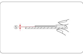
To check needle straightness, place the flat side of the needle onto something flat (a needle plate, glass etc.).
