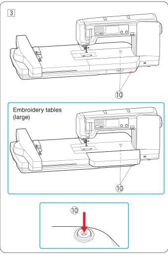
3 You can adjust the height of the embroidery tables to match the height to the top of the machine bed as necessary.
