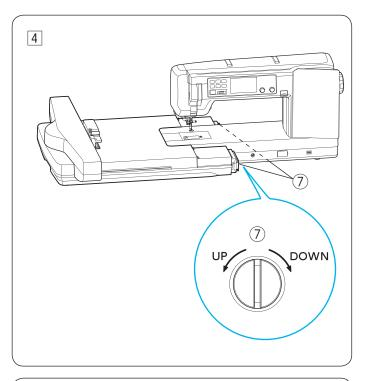
4 You can adjust the height of the embroidery unit to match the height to the top of the machine bed as necessary.
