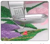
will strike before stitching begins for extreme precision. Perfect for designs that need to be placed in exactly the right position. Use the laser in conjunction with the baste function to ensure your design is where you want it.
