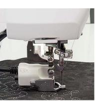
The A.S.R. (Accurate Stitch Regulator) foot holder reacts to the movement of the fabric and provides the same stitch length for free motion, ruler work, or variable zig zag quilting. We recommend thinking of this system as Free Motion Quilting (FMQ) training wheels. Training
