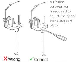
\*Remove the setscrew on the rear side of the spool stand and set the spool stand support plate in the correct position, as shown above.
