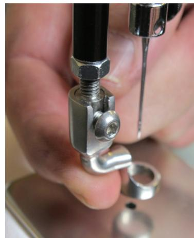
3. Fully tighten the screw with the 2.5 mm hex tool.
