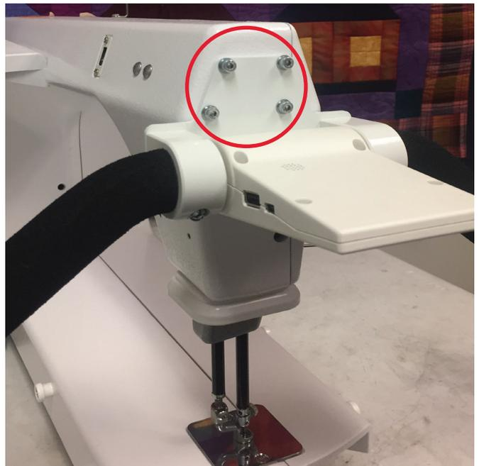
5. After the bolts are in place, plug the cable into the USB-style connection located on the front-left side of the machine. The upper small mini USB connection on the display is used to connect to the machine. The bottom regular USB connection on the right side of the display is for USB power only, no data.
