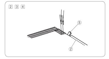
2 When you reach the next corner, stop the machine. Raise the needle and the presser foot.
