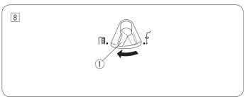
8 Return the looper threader switch lever to the "SEWING" position and close the looper cover.
