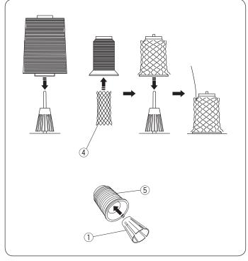
If the thread slips down from the spool during threading and/or sewing, put a net on the spool as illustrated to prevent jamming.
