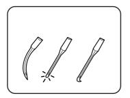
Insert a new needle into the needle clamp with the flat side to the back and push it up against the stopper, then tighten the needle clamp screw.
