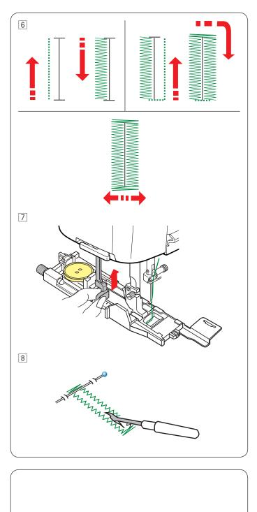
6 The buttonhole is sewn automatically in the sequence shown. When the buttonhole is finished, the machine will stop automatically with the needle in the up position. Press the thread cutter button and remove the fabric.
