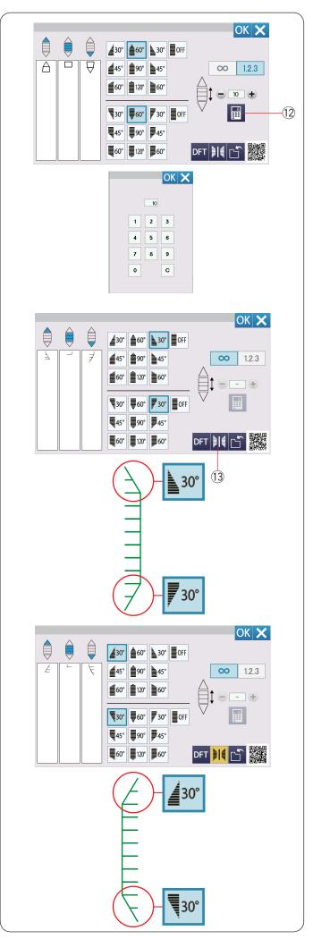
You can also set the number to repeat the pattern body by pressing the numeric pad key.
