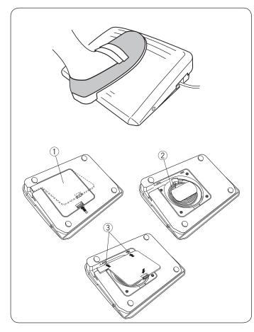
After sewing, depress the thread cutter switch 1 on the right side of the foot control to trim the both needle and bobbin threads.
