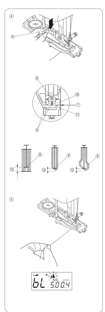
4 Lower the presser foot and pull the buttonhole lever down as far as it will go.
