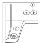
Raise the presser foot. Press the needle up/down button ① to raise the thread take-up lever to its highest position. ① Needle up/down button
