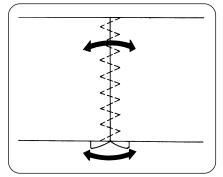
Sew seam and press seam allowance open. Sew pattern stitch on the right side of garment centering stitches over the seam line.
