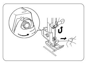
② Turn the handwheel slowly towards you with your right hand until the needle goes down and continue turning handwheel until the take-up lever is at its highest position.
