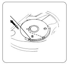
Continue to draw the thread lightly until the thread slips into notch **B**.
