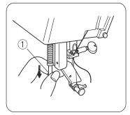
Raise the needle to the heighest position. Lower the presser foot.
