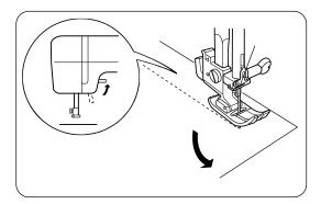
Stop the machine and bring the needle down into the fabric by turning the handwheel.
