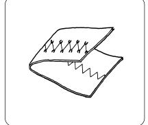
To obtain better zigzag stitches, the needle thread tension should be slightly weaker than in the case of straight sewing. The needle thread should appear slightly on the reverse side of the fabric.
