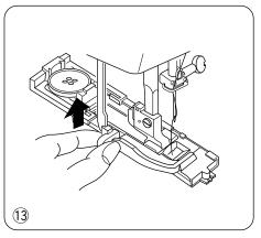
(3) When buttonhole sewing is finished, push the buttonhole lever upward as far as it will go.
