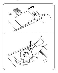
Gently slide the hook cover plate release button to the right, and remove the cover plate.
