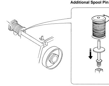
The additional spool pin is used to wind extra bobbins without unthreading the machine. To use, insert the additional spool pin in the hole. Place the felt and the spool on the pin.
