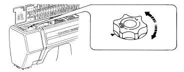
The pressure dial should be set at "3" for regular sewing. Reduce the pressure to "2" for appliques.
