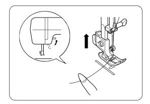
1 Raise the presser foot and hold the needle thread lightly with your left hand.
