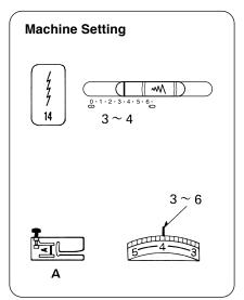
Pattern 14 is a narrow stretch stitch designed to eliminate puckering on knit fabrics and bias seams, while permitting the seam to be pressed completely flat.
