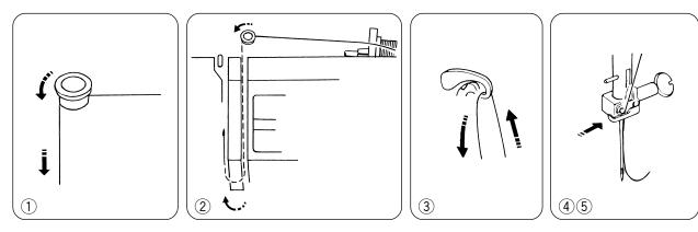
Raise the take-up lever to its highest position by turning the handwheel toward you.
