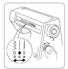
Select the pattern by turning the pattern selector dial and the red signal shows the selected pattern.
