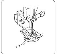
Align the both holes of button with the needle swing, lower the foot and depress the foot control.
