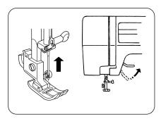
Turn the handwheel toward you to raise the needle to its highest position. Raise the presser foot.
