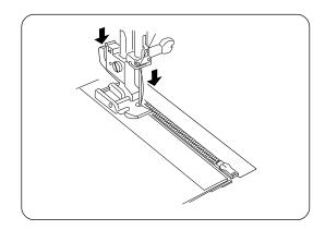
Attach the zipper foot with the pin on the right hand side. Lower the zipper foot.
