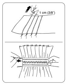
With the stitch length control at "4", sew straight lines 1 cm(3/8") apart across the area to be smocked. Knot the threads along the ege. Pull the bobbin threads and distribute gathers evenly. Sew pattern stitches between the straight seams. Pull out the gathering stitches.
