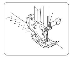
foot so that the edge will be slightly inside the right hand side of the presser foot.
