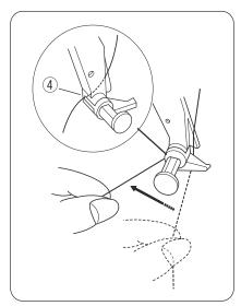
Draw the thread to the left into the groove on the back.
