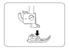
When attaching the presser foot, the pressure dial should always be at position "3".
