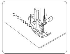
Simple zigzag stitch is widely used for overcasting, applique, sewing on buttons etc.
