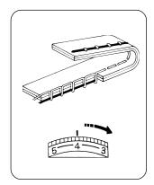
Tighten the needle thread tension by moving the dial to a higher number.
