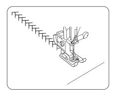
Sew a row of stitches and adjust the thread tension so the needle thread should appear on the reverse side of the fabric.
