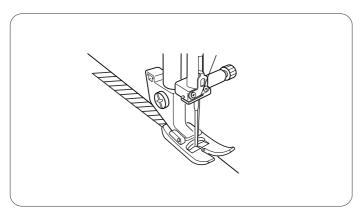
This stitch is ideal for 1/4" (0.6 cm) seams on knits or on medium to heavy weight woven fabrics where you want a narrow seam. It is also great for sewing spandex swim wear. Place the fabric under the presser foot [A] so that the stitches are made over the raw edge.
