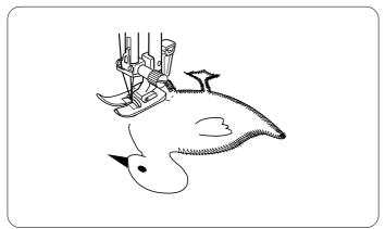
Baste applique pieces on the fabric, or fuse the applique pieces with iron-on fabric joiner. Stitch around the applique making sure the needle falls along the raw edge of the applique.
