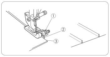
Fold the fabric wrong sides together and lower the needle into the fabric 0.1 - 0.2 cm inside the folded edge.
