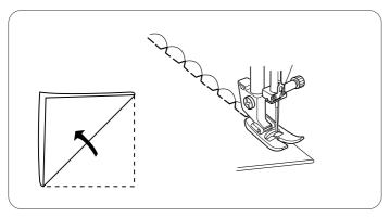
Use a lightweight fabric (tricot, for example). Fold the fabric in bias and stitch on the fold. Allow the needle to just clear the folded edge to create a shelled edge. You may need to increase the needle thread tension slightly.
