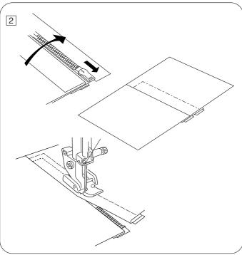
2 Raise and release foot, and re-attach it on left-hand side of pin.
