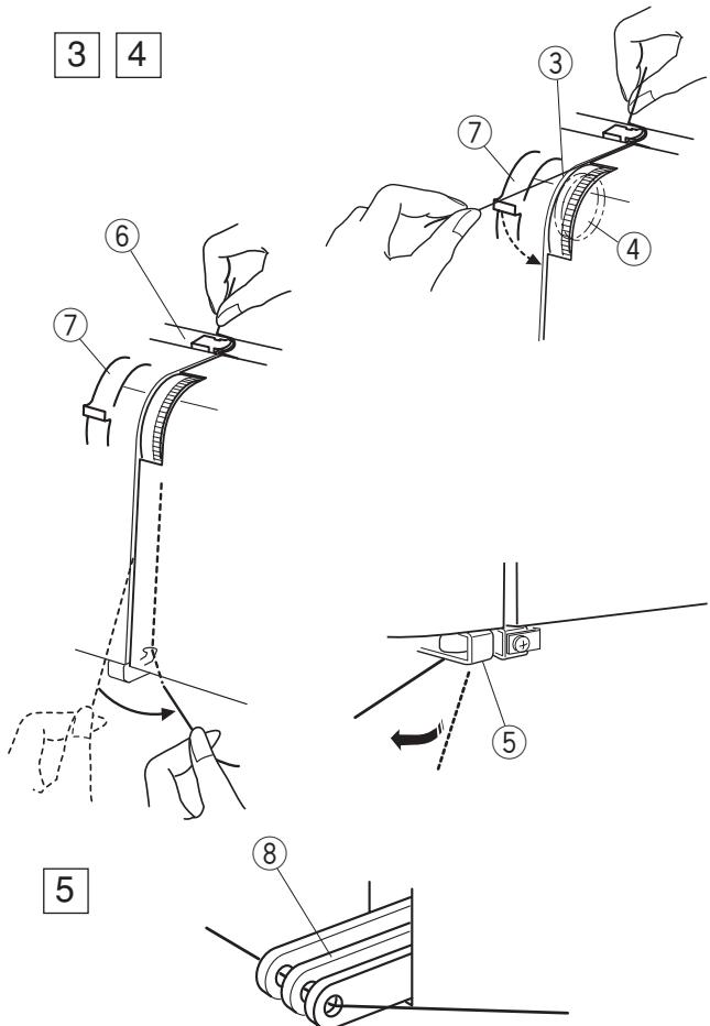
③ Hold the thread at both ends and tug gently to ensure the thread is correctly inserted between the tension disks. (If the presser foot lifter is raised, the thread easily inserts between the tension disks.)
