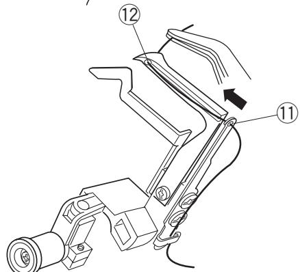
⑧ Pass the thread through the eye of the looper thread guide (D) then through the eye of looper.
