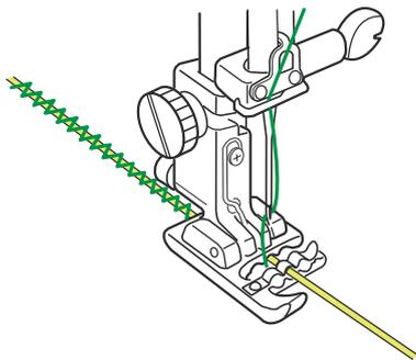
For a single strand cording, insert a strand into the center groove on the foot.
