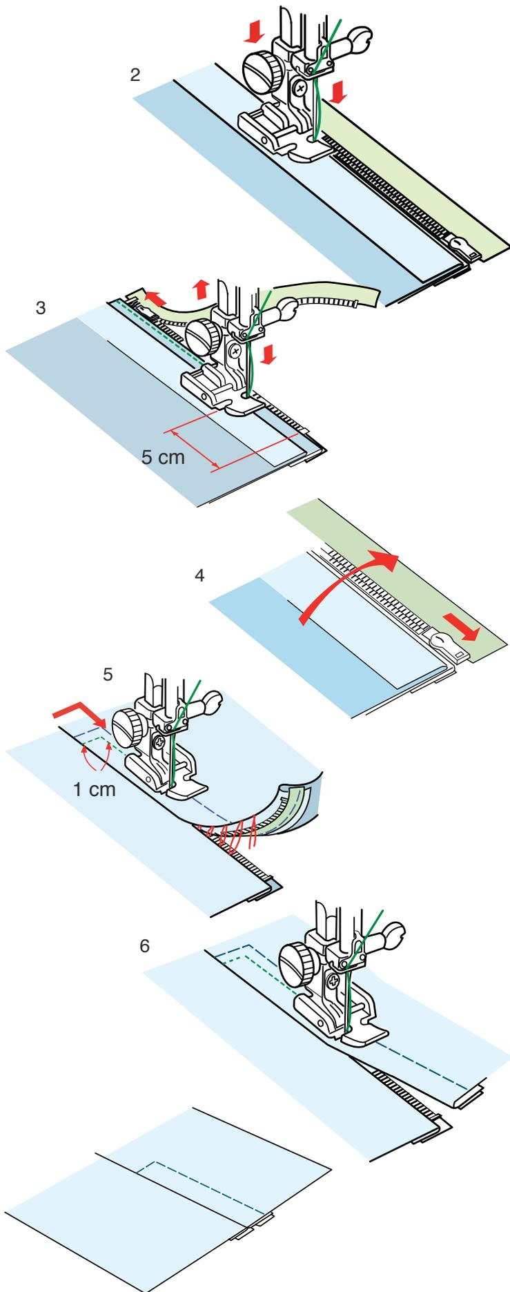
2. Attach zipper foot E with the pin on the right hand side. Lower the foot onto the topside at the bottom of the zipper so that the needle pierces the fabric next to the fold and the zipper tape. Sew along the zipper guiding the zipper teeth along the bottom edge of the foot.
