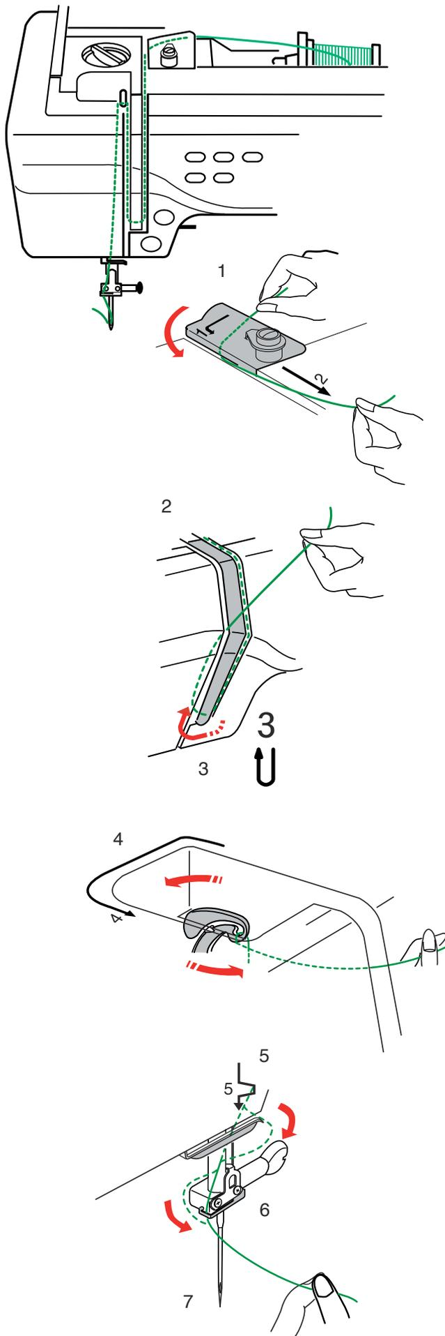
1 Draw the thread from the spool. Hold the thread with both hands and pass the thread under the thread guide plate. Tug the thread until it snaps.
