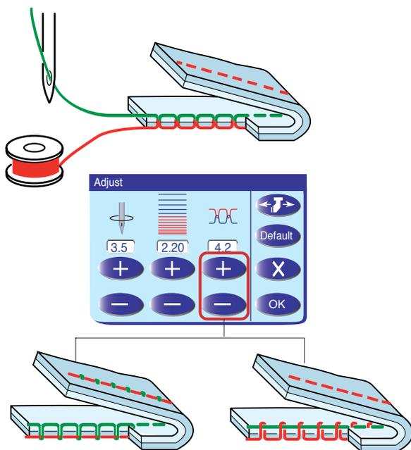
This machine is equipped with automatic thread tension control, however you may need to manually adjust the tension balance depending on the sewing condition, or you can fine-tune the thread tension to suit your preference.
