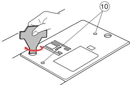
7. Reattach the needle plate, aligning the guide holes on the needle plate with the needle plate guide pins and tighten the screw.
