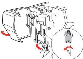
If the automatic needle threader will not return to the up position by pressing the auto needle threader button, correct it as follows:
