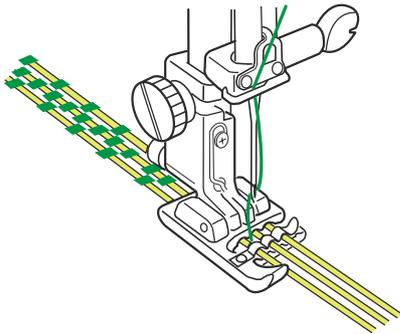
Pull 10 cm (4") of strands under the foot and to the rear. The grooves on the bottom of the foot will hold cordings in place while stitching over the cordings.
