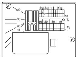
You can seam patchwork pieces at the desired angle without marking, by using the angle scale on the needle plate.
