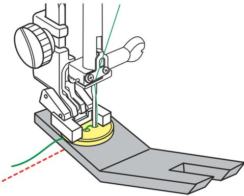
Place a button on the fabric and lower the needle into the left hole of the button by turning the handwheel with your hand.
