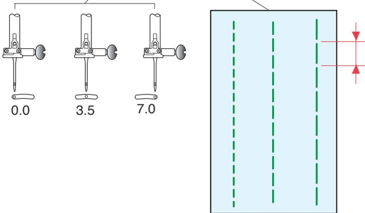
Press the “+” key to move the needle drop position to the right.
