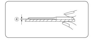
To check needle straightness, place the flat side of the needle onto something flat (a needle plate, glass etc.) The gap between the needle and the flat surface should be consistent. Never use a blunt needle. ④ Gap
