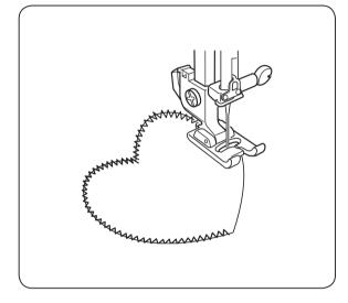
Baste appliqué pieces on the fabric, or fuse the appliqué pieces with an iron-on fabric joiner. Stitch around the appliqué, making sure the needle at the right swing falls along the outer edge of the appliqué.
