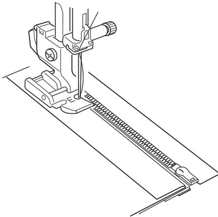
2 Attach the zipper foot E with the pin on the right hand side.
