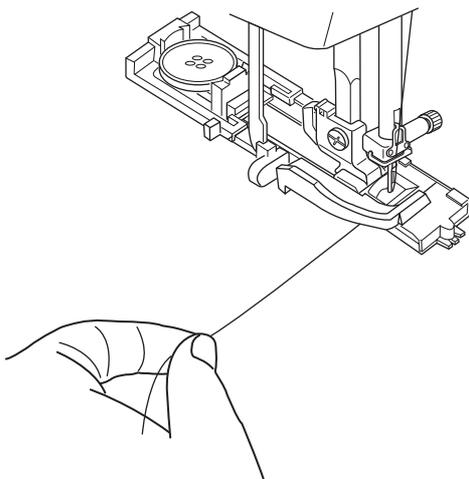
5 Start sewing while pulling the needle thread lightly to the left. After sewing a few stitches, free the thread and continue sewing.
