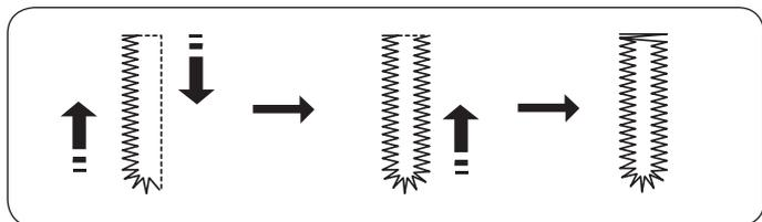
Sewing procedure is the same as square buttonhole. The buttonhole width can be varied from 2.5 to 5.5. The stitch density can be varied from 0.2 to 0.8.
