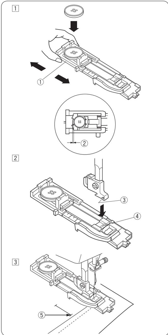
The size of a buttonhole is automatically set by placing a button in the rear of automatic buttonhole foot R. The button holder of the foot takes a button size of 1 cm (3/8") to 2.5 cm (1") in diameter. When selecting the buttonholes, the LCD screen advise you to lower the buttonhole lever.
