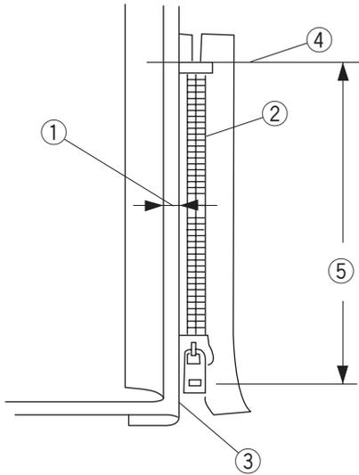
1 Fold back the left seam allowance. Turn the right seam allowance under to form a 0.2 to 0.3 cm (1/8") margin. Place the zipper teeth next to the fold and pin in place. Set the stitch length and thread tension back to the original setting.
