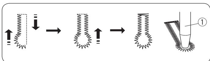
Sewing procedure is the same as square buttonhole. The buttonhole width can be varied from 5.5 to 7.0. The stitch density can be varied from 0.3 to 0.8. Use the seam ripper and an eyelet punch to open the buttonhole.
