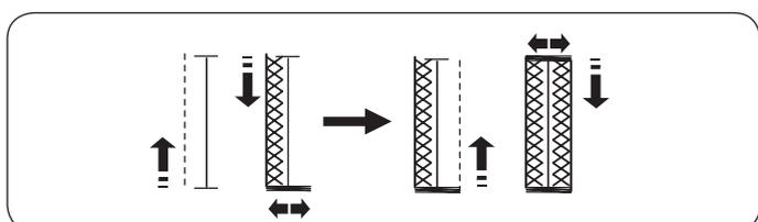
The machine will sew the front bartack and left row first. The machine will sew the back bartack and right row, then it stops automatically. The stitch width can be varied from 2.5 to 7.0. The stitch density can be varied from 0.7 to 1.2.
