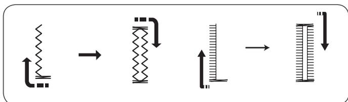
The machine will sew the front bartack and left row first. The machine will sew the back bartack and right row, then it stops automatically. The stitch width can be varied from 2.5 to 7.0. The stitch density can be varied from 0.5 to 1.0 (Stretch buttonhole), 0.5 to 2.5 (Antique buttonhole).
