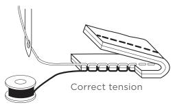
Conversely, if the thread is looping on top, make sure the bobbin thread is coming off the bobbin counterclockwise and that the thread is securely threaded in the bobbin tension guide.
