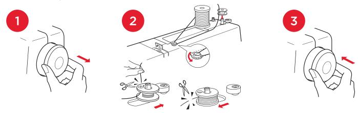
In order to ensure correct bobbin winding, follow the above diagram for correct threading. Use both hands to thread machine around the guide for correct tension.
