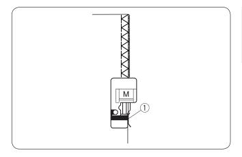
This stitch is excellent for sewing fabrics that tend to fray extensively such as linens and gabardines. Two rows of zigzag stitches are simultaneously sewn over the edge to insure that your seams will not ravel. Sew while guiding the fabric edges along the guide on the foot.
