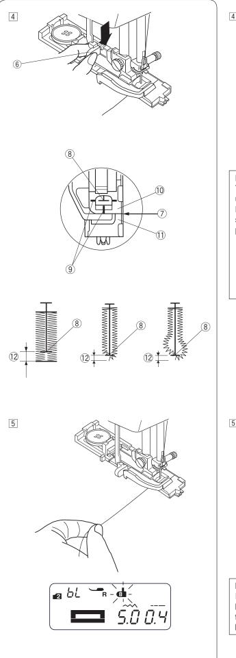
4 Lower the presser foot and pull the buttonhole lever down as far as it will go.
