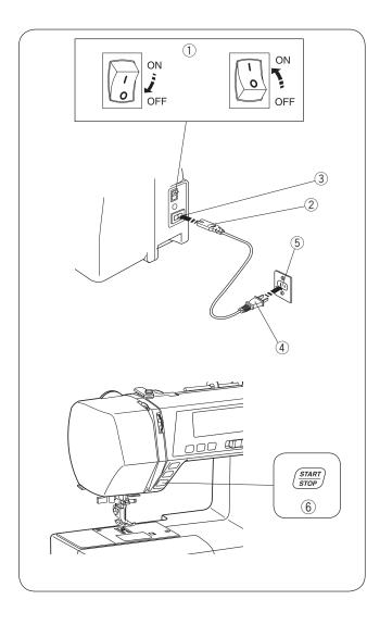
Using the start/stop button Turn off the power switch. Insert the machine plug into the power inlet. Insert the power supply plug into the wall outlet. Turn on the power switch.
