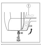
Raise the presser foot. Press the needle up/down button 1 to raise the thread take-up lever to its highest position.
