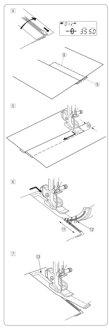
4 Close the zipper and spread the fabric open flat with the right side facing up. Attach the Zigzag foot A.
