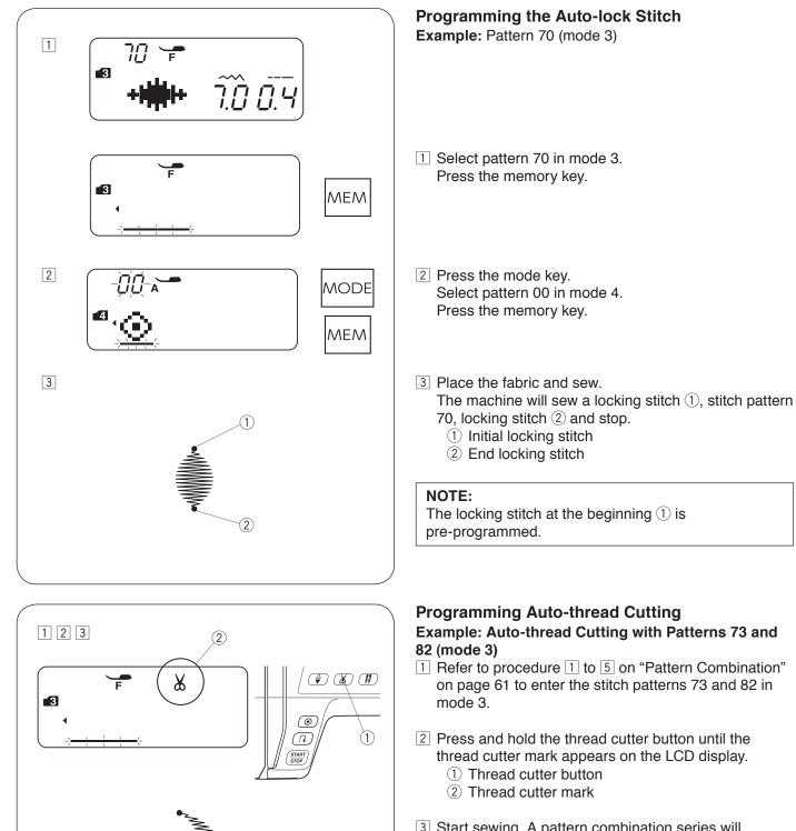
3 Start sewing. A pattern combination series will be sewn and the machine will trim the threads automatically after locking stitch.
