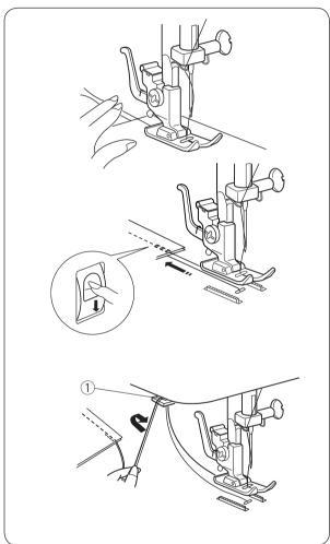
1 Raise the presser foot and position the fabric with its edge lining up with a seam guide line on the needle plate.
