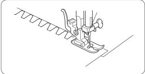
Use this stitch to join heavy weight fabrics. Overlap two raw edges together and use this stitch to join them.
