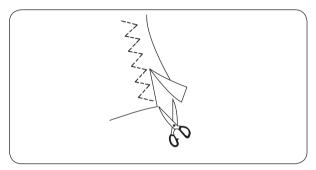
This stitch is used to finish the raw edge on synthetics and other fabrics that tend to pucker. Place your fabric to allow a 1.6 cm  $(5/8^{\circ})$  seam. Trim the seam allowance after sewing. Be careful not to cut the stitches.
