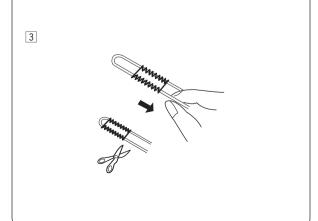
3 Remove the fabric from the machine and cut the sewing threads.
