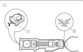
With the buttonhole foot raised, hook the filler cord on the cord spur at the back of the buttonhole foot.
