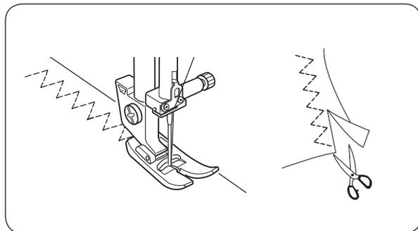
This stitch is used to finish a raw edge on synthetics and other fabrics that tend to pucker. Place the fabric to leave a 5/8" (1.6 cm) allowance. Trim the extra allowance after sewing.
