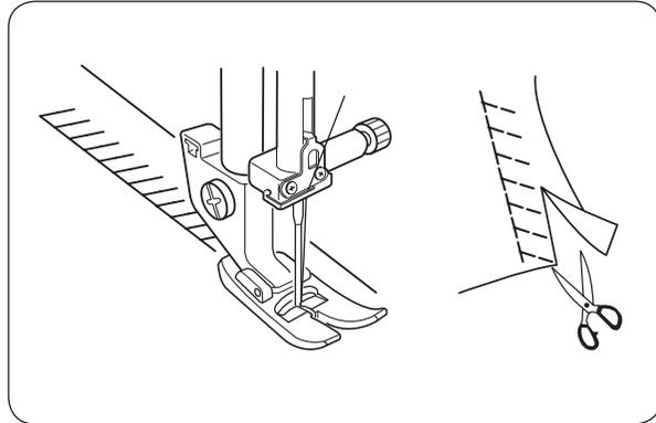
This knit stitch is ideal for sewing swimwear and stretch velour because it provides the greatest amount of elasticity and strength. Place your fabric to allow a 5/8" (1.6 cm) seam. Trim the seam allowance after sewing.
