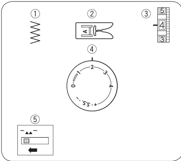
Unthread the needle. Adjust the stitch width to match it with the span of the holes in the button. Turn the handwheel to check if the needle enters into each hole in the button.
