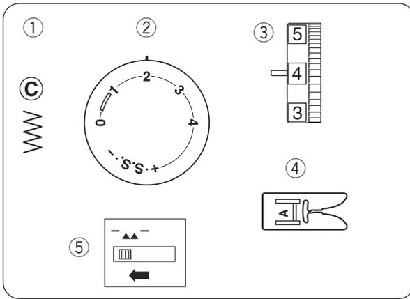
Unthread the needle. Adjust the stitch width to match it with the span of the holes in the button. Turn the handwheel to check if the needle enters into each hole in the button. Lower the foot to hold the button in place. The holes in the button should align with the slot of the foot.
