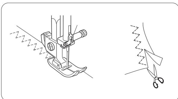
This stitch is used to finish a raw edge on synthetics and other fabrics that tend to pucker. Place the fabric to leave a 5/8" (1.6 cm) allowance. Trim the extra allowance after sewing. It is also used for mending tears.
