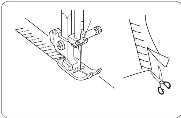
This stitch is ideal for 1/4" (0.6 cm) seams on knits or on medium to heavy weight woven fabrics where you want a narrow seam. It is also great for sewing spandex swim wear. Place the fabric to leave a 5/8" (1.6 cm) allowance.
