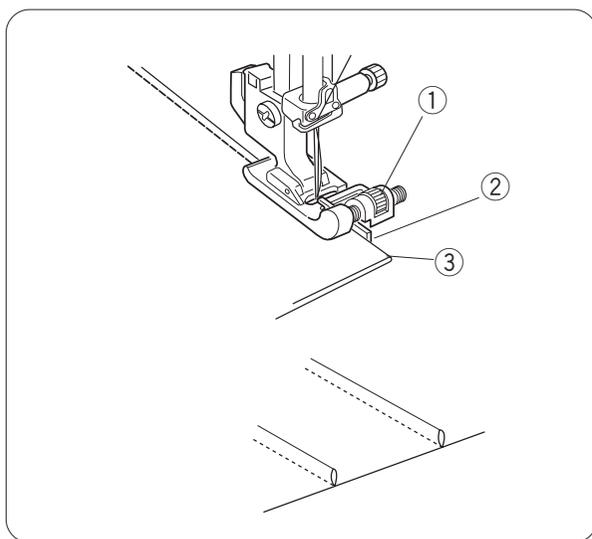
Fold a fabric wrong side together and Lower the needle into the fabric 0.1 – 0.2 cm inside the folded edge.
