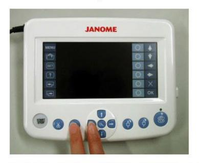
Be sure to keep the buttons pressed for at least 3 seconds until the LCD screen shows the pale blue background.
