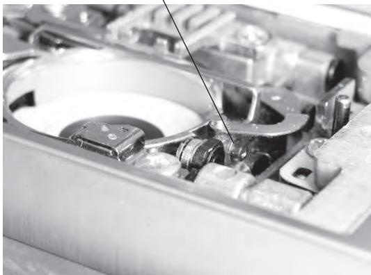
1. Remove the presser foot, the needle plate and the bobbin holder. (see page 4)
